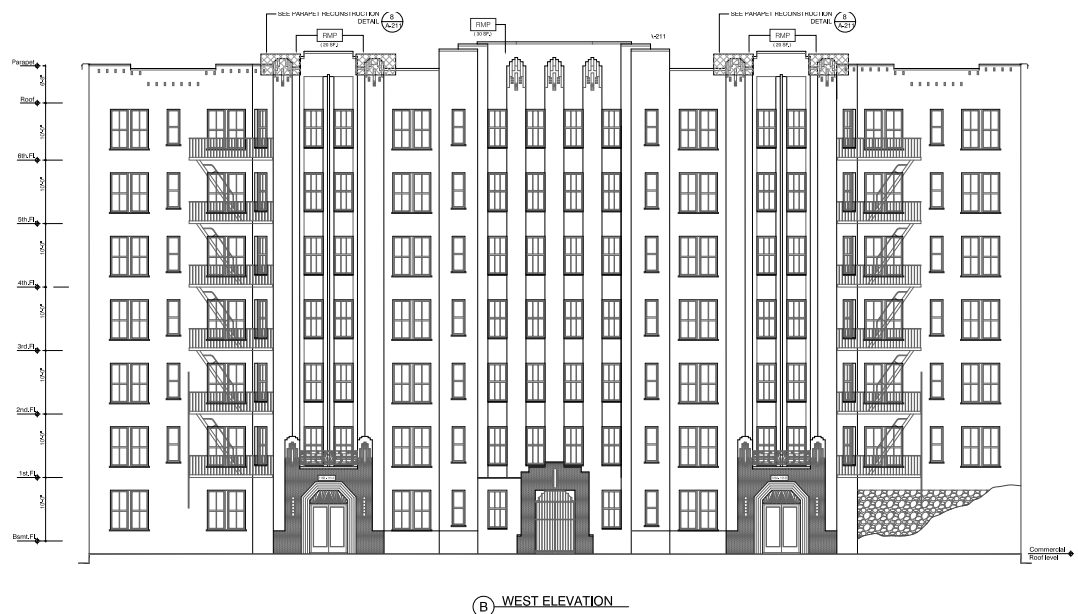
Figure 12. Interior west elevation, with view from the "garden court" in which the intervention areas of the parapet are indicated. The notes identified as RMP indicate the areas of the parapet where restoration work was carried out. Source: Danois Architects, P. C. (2020)
