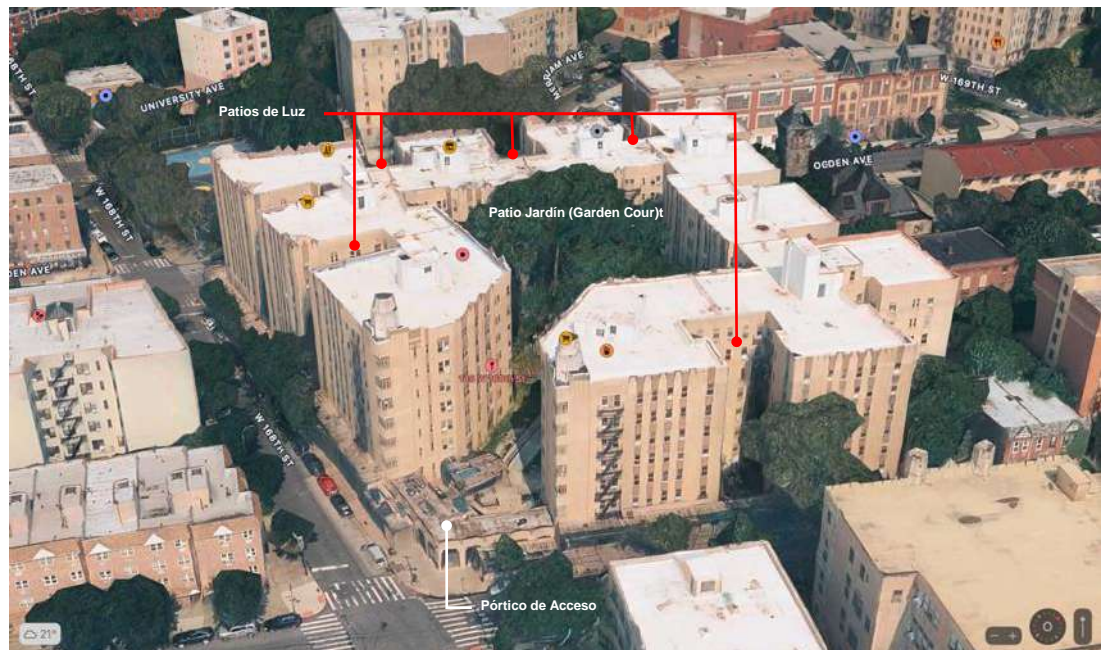
Figure 14. Infographic showing the tree planting of the "garden court", the volumetric joints produced by the lighting courts, which contribute to ventilation and natural lighting and generate a rhythm that breaks with the frequent monotony of large high-density housing blocks. Source: Prepared by the author (2023), on three-dimensional cartography taken from the Apple Inc Maps application.
